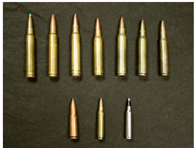
Figure 10. Big game hunting and military ammunition are high velocity and designed to retain bullet stability for delivering major destructive kinetic energy at longer distances. The top row is typical big game hunting ammunition, ranging on the left a 300 Weatherby magnum to the right a 30.06 Springfield. On the bottom row is typical military ammunition, on the left, an AK47; the middle, an M-4; and the right, an AR15 with a Teflon jacketed bullet.
