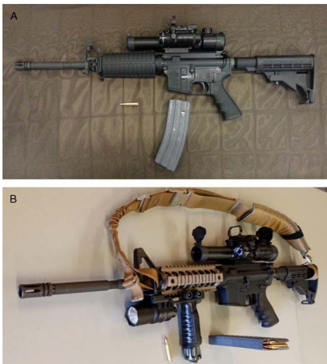
Figure 11. A, Semiautomatic assault rifle with adjustable stock, scope, heads up sighting system, and laser targeting device. B, Same rifle with a different handguard, lighting system, and sling.
